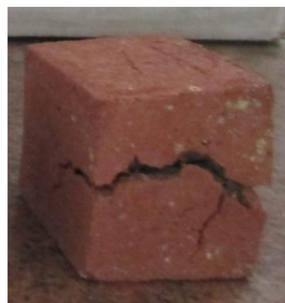
Fig (6): Apparent crack formation in sample containing 20% waste fired at 850°C
